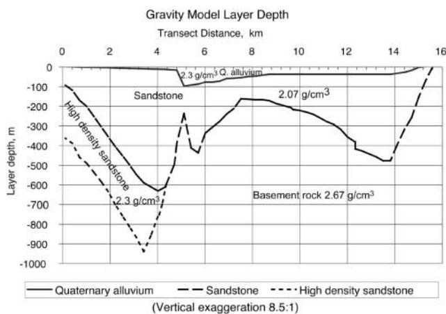
Figure 2. Depth-of-alluvium and depth-to-basement-rock profile for points along our transect (Fig. 1) from the gravity model of Abbott and Louie (2000). The densities of each rock unit used in modeling are shown. Refer to Figure 1 for geographical reference of transect distances.
