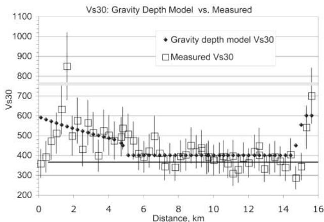
Figure 8. Vs30 according to an alluvium-depth model derived from a basin-gravity survey (Abbott and Louie, 2000) versus the measured values of Vs30 along the transect with  $\pm 20\%$  error bars on the measurements.
