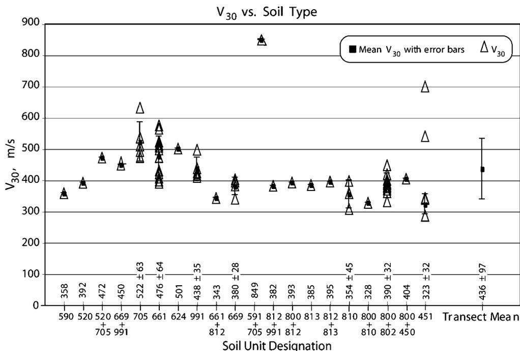
Figure 7. Measured values of Vs30 versus soil-type designations (Table 2). Most individual units have just one Vs30 measurement and thus no deviation. The velocity average and standard deviation of the other units are indicated. Units are combined where an array measurement overlaps both.
