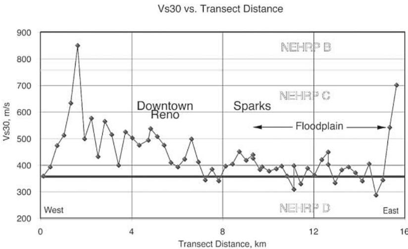
Figure 4. Our measured values of  $V_{s30}$  for 55 points along the Reno transect.  $V_{s30}$  values are slowness-averaged from 55 modeled velocity–depth profiles. Sites with  $V_{s30}$  greater than 760 m/sec are classified as NEHRP B; between 760 and 360 m/sec, as NEHRP C; and 360 to 150 m/sec, as NEHRP D (plot extends only to 200 m/sec). Refer to Figure 1 for geographical references for transect distances.
