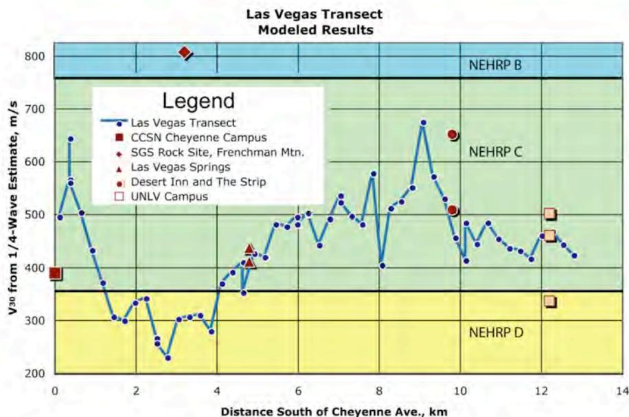
Fig. 3: Depth-averaged values of  $V_{s30}$  for 49 points along the Las Vegas transect.  $V_{s30}$  values are slowness-averaged from 49 modeled velocity-depth profiles. Eighteen of the transect locations were independently modeled by different analysts; all of the values they obtained are plotted. Refer to fig. 1 for geographical reference for transect distances.  $V_{s30}$  values obtained by various techniques at sites off the transect are also plotted after projection onto the transect.
