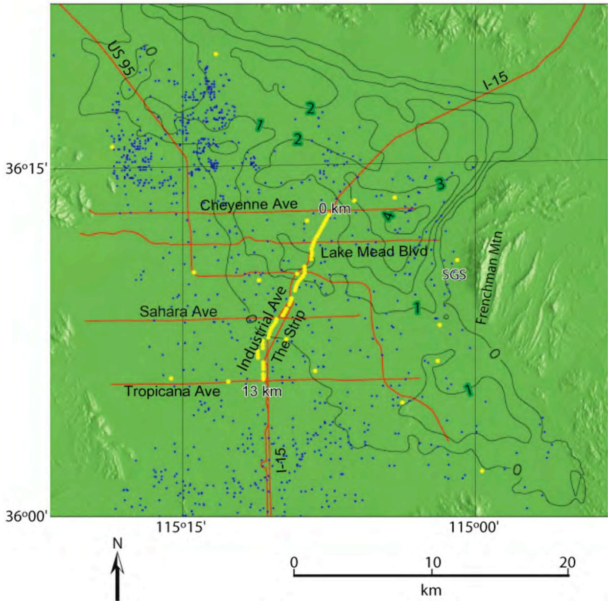
Fig. 1: Map showing the location of our transect across the Las Vegas, Nevada urban basin. Yellow dots mark the locations of Vs measurements and blue dots mark the locations of the wells used to provide stratigraphic data. Basin depths (one km contours) are from Langenheim et al. (2001). Transect distances at ends are indicated.
